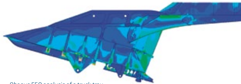
Abaqus FEA analysis of a truck tray.
