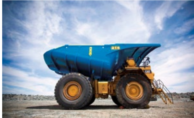
The dump truck tray extends over the driver's cab and can be as long as the entire vehicle.
