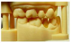
Die inserted in quadrant model EnvisionTEC 3Dent™ (antagonists placed together) with precise position of die and coping in quadrant model (one precise system):
