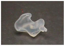
Traditional processing meant an impression of the ear was taken, from which the sculptor had to make a positive of the ear to pour plastic into. Once this was done the whole project was cured in ultraviolet light to get a plastic piece. This plastic piece still had to be drilled for vents and sound holes or general additional manual processing to acheive the final shape.
