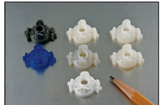
This image shows challenge parts. Top row (left to right): Perfactory MML, Fortus 200mc, and Dimension Elite. Middle row (left to right): ProJec HD3000, Alaris 30, and Eden260 V. The molded part is in the bottom row.
