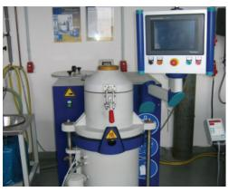
The flask is then blown out with compressed air and vacuumed, the metal is poured and the mould allowed to cool.
